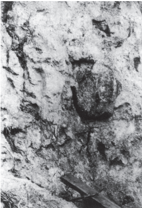
Figure 2. Pipe around corestone in weathered granodiorite
